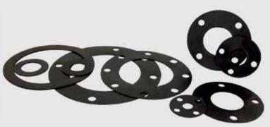
We offer a wide range of elastomeric gaskets which consist of base polymers with the insertion of vulcanizing agents, fillers, pigments and various additives. They have relatively soft compression characteristics, which ensure excellent recovery properties due to their self energizing behaviour.
